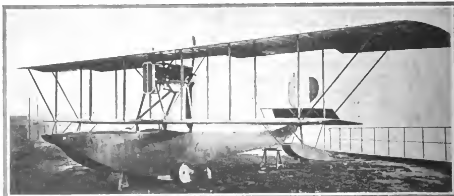
An Hispano-Suiza hydro-aeroplane which has an eight cylinder aluminum engine with a special valve mechanism
